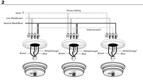
\* Interconnect only - if single alarm installation, leave unconnected with sheathing intact.
