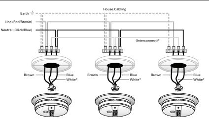
\* Interconnect only - if single alarm installation, leave unconnected with sheathing intact.
