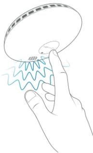
**EN** You should test the smoke detector every month to ensure that it is properly installed and working correctly. You can carry out the test directly on the detector by pressing the central button for three seconds. Note that the alarm will sound for eight seconds. If the alarm does not sound, either the battery is defective or there is another fault (see Troubleshooting on pages 12-13). Do not use a flame due to the risk of damaging the detector.
