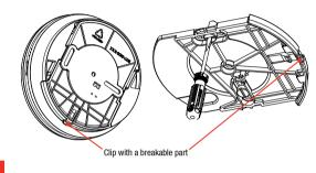
The alarm must be fixed horizontally and to the ceiling using the enclosed mounting plate. The mounting plate can be screwed to the ceiling using either the central hole or the two slots in the ceiling mounting plate (see diagram).
