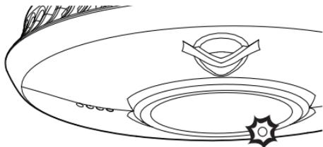
**NOTE:** The test button accurately tests the alarm's smoke sensing circuit, there is no need to test your alarm with smoke. If your smoke alarm fails to give an audible test signal, please refer immediately to the trouble shooting guide at the end of this manual.
