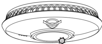
**NOTE:** The test button accurately tests the alarm's smoke sensing circuit, there is no need to test your alarm with smoke. If your smoke alarm fails to give an audible test signal, please refer immediately to the Troubleshooting section at the end of this manual.
