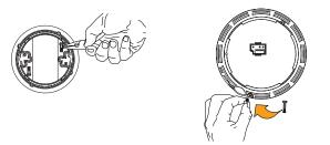
3. Push the locking pin through the hole near the battery drawer on the back of the Smoke Alarm.
